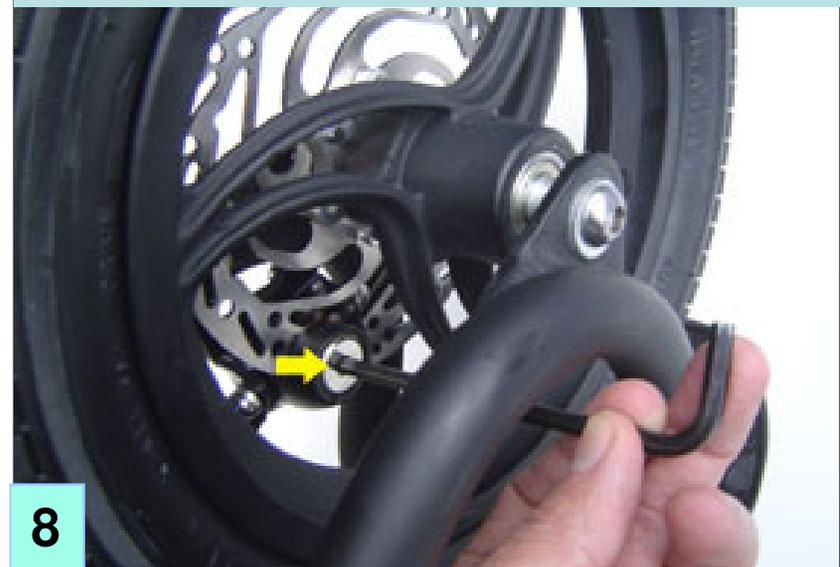
Re-tightening the lateral caliper bracket bolts by alternating several times from bolt to bolt. Don't tighten one then the other.
