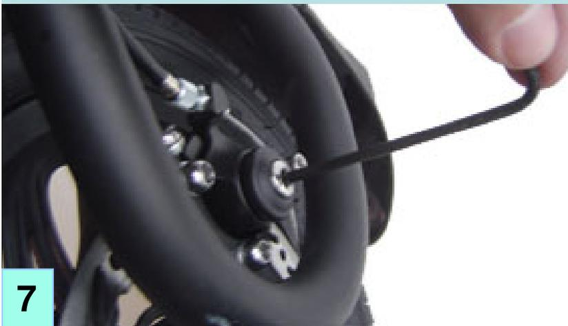
Using a 5mm allen wrench, tight the inner pad against the disc until the disc is locked. You should not be able to rotate the wheel.
