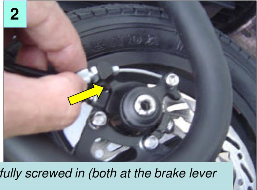
The brake cable adjustment screws must be fully screwed in (both at the brake lever on the handlebar and at the brake caliper).
