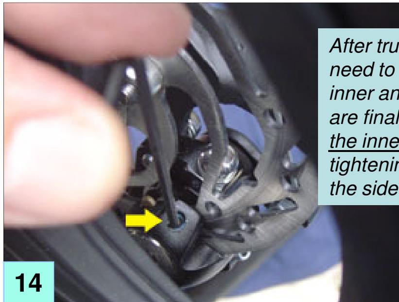
*After trueing the discs in step 13, you might need to make minor adjustments to the inner and outer pads. When adjustments are final, use a 2.5mm allen wrench to lock the inner pad adjustment screw by tightening its locking bolt ( a small bolt at the side of the inner pad body)*
