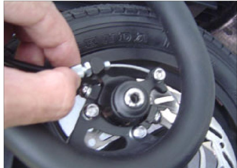
After some use, the brake pads will wear down a bit and seat properly with the disc. Also, the brake cable will stretch. Re-adjust your brakes using the fine adjustment screws at the brake lever and at the caliper as seen in steps 1 & 2.
