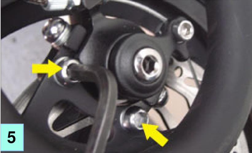
Loosen the 2 lateral bolts that connect the caliper to its bracket (not to the trikke frame), using a 5mm allen wrench. Loosen them well...
