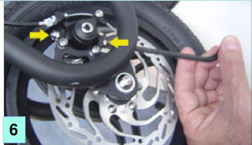
Using a 3mm allen wrench, back the outer pad away from the disc until it stops.
