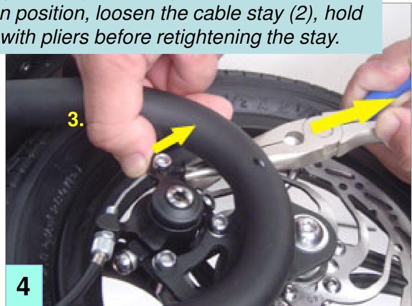
Make sure the two bolts that connect both calipers to the frame are tight.
